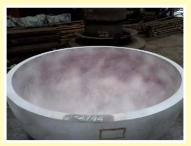
Dished End - Mfgd. at Mulund Unit Size: - 1375 mm i/d x 80 mm thk Client: Thermax Ltd., Pune
