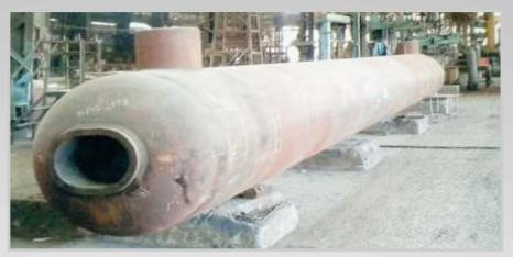
Mfgd.By R&C (1972) Ltd:-Byculla Unit Fabrication of Water Drum Size: 63mm Thk x 960 mm I/D x 10725 mm Long Client:-M/s.Sitson India Pvt. Ltd.
