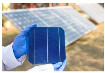
Prototype high efficiency solar cell using PERC technology under development at BHEL ASSCP, Gurugram
