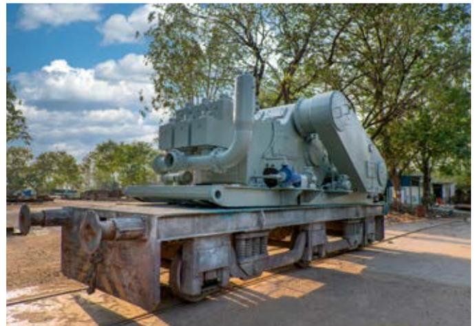
*Mud pump used in oil rig system ready for dispatch at HPEP Hyderabad*
