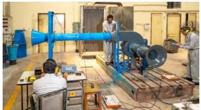
*Axial fan speed and flow test facility at Corporate R&D, Hyderabad*
