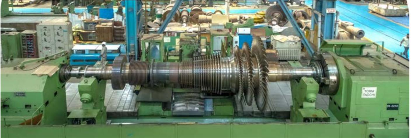
*Highest rating 150 MW IP turbine for captive plant applications at under testing at HPEP Hyderabad*
