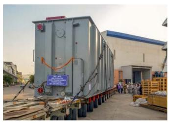
295.1 MVA, 800 KV, HVDC CONVERTER TRFR for 800 kV Class Single phase HVDC Converter Transformer being despatched from HEP Bhopal
